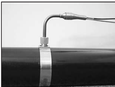
Fig. 3 Proper installation of EGT sensor
